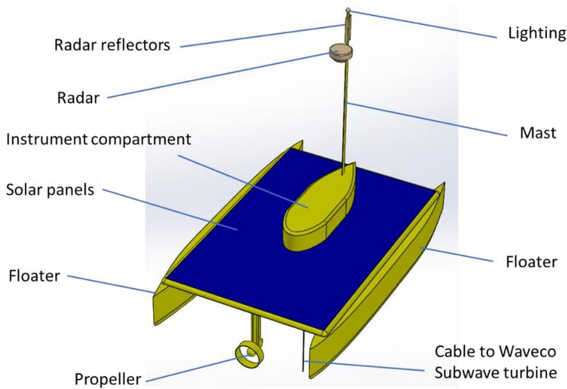
*Figure 1: Scheme of the catamaran type of self positioning platform*
